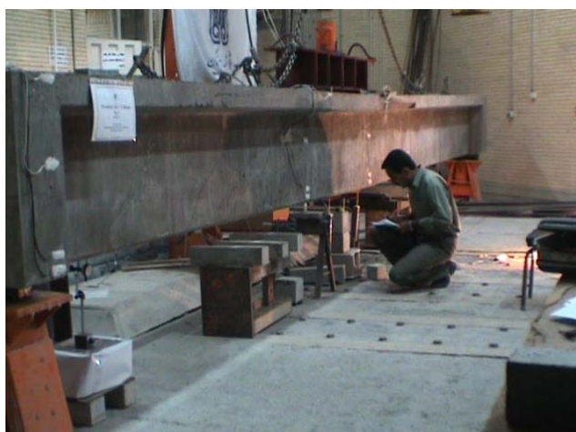
Figure 1- Loading arrangement and position of gauges on beam[7]
