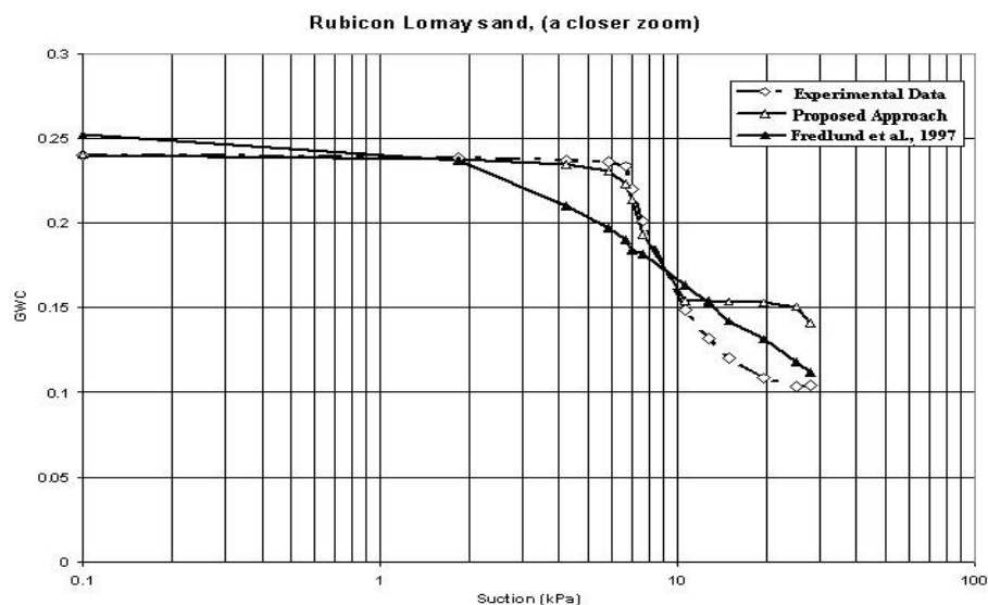
Figure 8– Simulated and experimental SWCC curve for Rubicon loamy sand (soil #63 of soil Vision)
