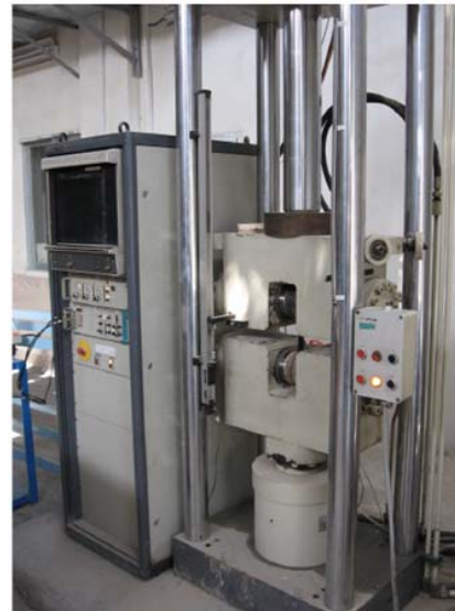
Figure 3– Tension test set-up
