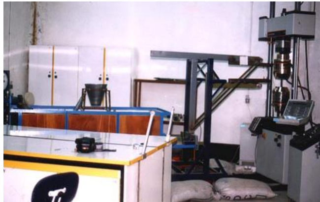
Figure 3 – Lateral view of arraying the Servo-Hyd. , xformer and pipe, soil and box system
