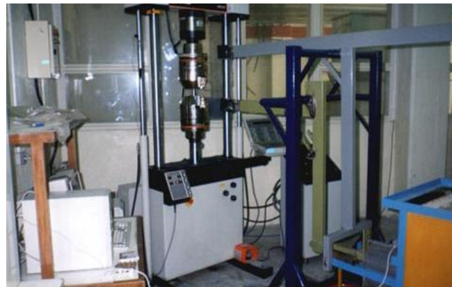
Figure 4 – General view of arraying the Servo-Hyd. , xformer and base and computer system
