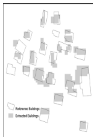
Fig. 4. Examples of extracted polygons and reference buildings.
